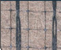
Created with three UV-stabilized nets, the three dimensional ECC-3 will provide protection through all phases of vegetation growth. The layer of coconut fiber is slow to degrade and helps with the germination. This is an excellent choice for high-flow areas and steep embankments where a permanent solution is needed.
