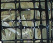
Designed to provide erosion protection necessary for the establishment of vegetation, and provide a permanent solution for turf reinforcement, the ECSC-3 is highly suited for use in high-flow channels, lakes, ponds, or other high-flow areas. A permanent, three layer netting structure firmly helps secure establishing roots, while including the benefit of the straw/coconut matrix blend.
