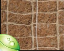
Ideally suited for erosion protection and the establishment of vegetation up to 24 months, the ECC-2B is an erosion blanket designed for steep embankments exceeding a 1:1 grade and moderate channel flow. The blanket is slow to degrade, providing the most extended temporary erosion control available.
